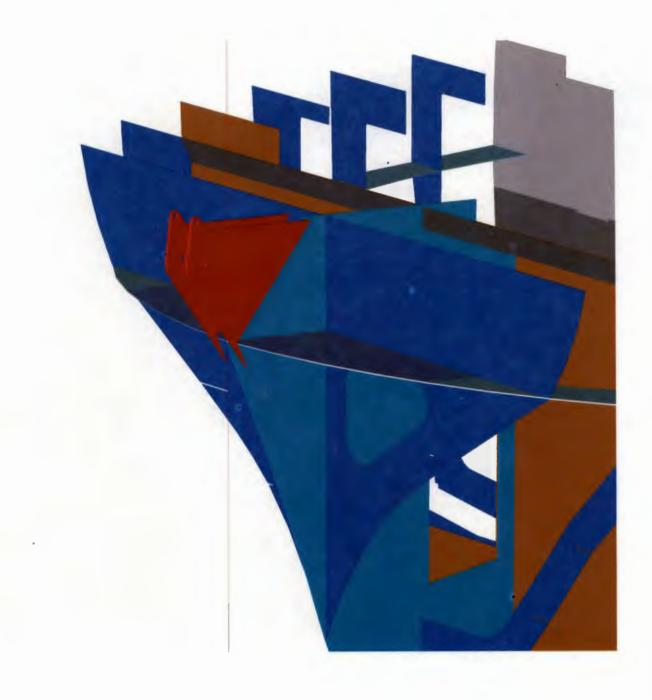
4. Deck plating (gray color) is added behind station 1 as roof to accommodate the needed head room in the below deck sleeping quarters.
