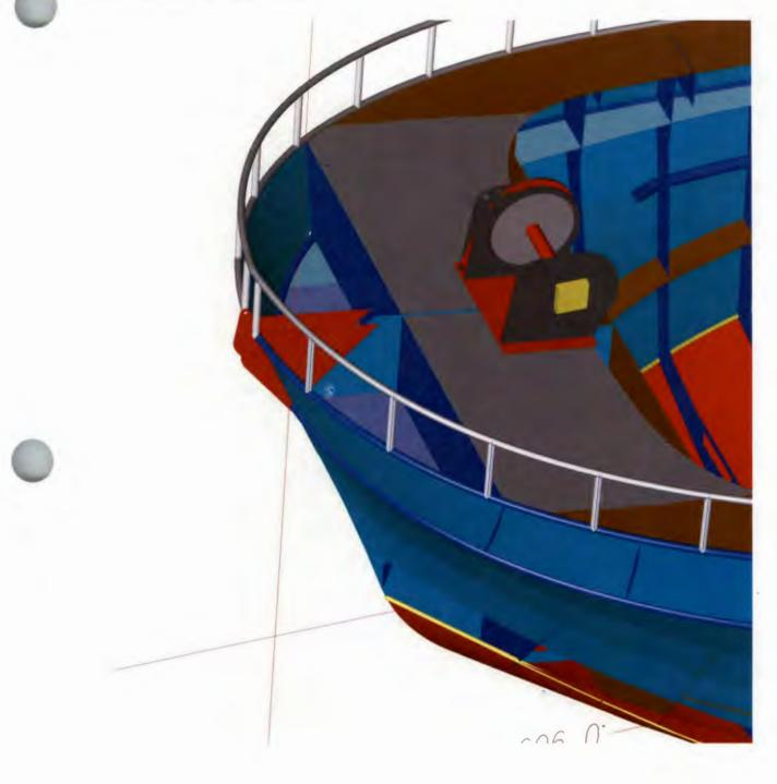
5. hull plating and forward bulwarks are wrapped around the frames and solidly welded into the bow roller and bow stem creating a buoyant envelope that is still 58' long.
