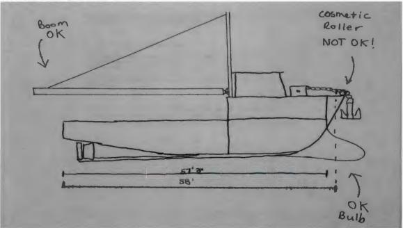
It is currently acceptable to exceed the 58' rule just not on the upper half of the front of the vessel.
