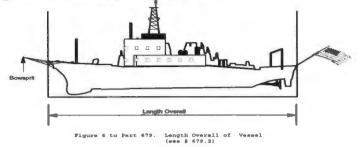
**LOA:** the horizontal distance of the hull between the foremost part of the stem and the aftermost part of the stern, excluding anchor rollers.
