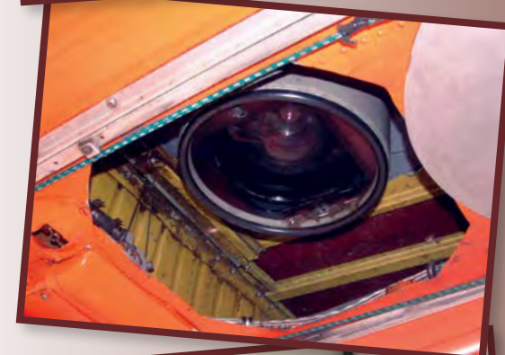
A mapping camera is mounted in the belly of the plane.
